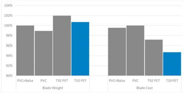
Fig. 3: Blade weight and blade cost differences based on STRUCTeam's 80m reference blade, STL80-6MW
