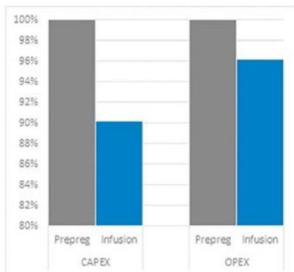
Fig. 1: CAPEX and OPEX cost difference based on STRUCTeam's 80m reference blade, STL80-6MW
