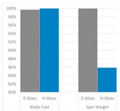
Fig. 2: Blade cost and spar cap weight differences based on STRUCTeam's 80m reference blade, STL80-6MW
