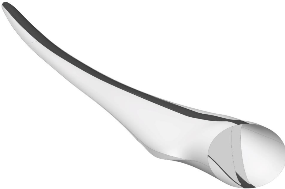
STL785C – STRUCTeam 80m Blade design deploying carbon spar caps
